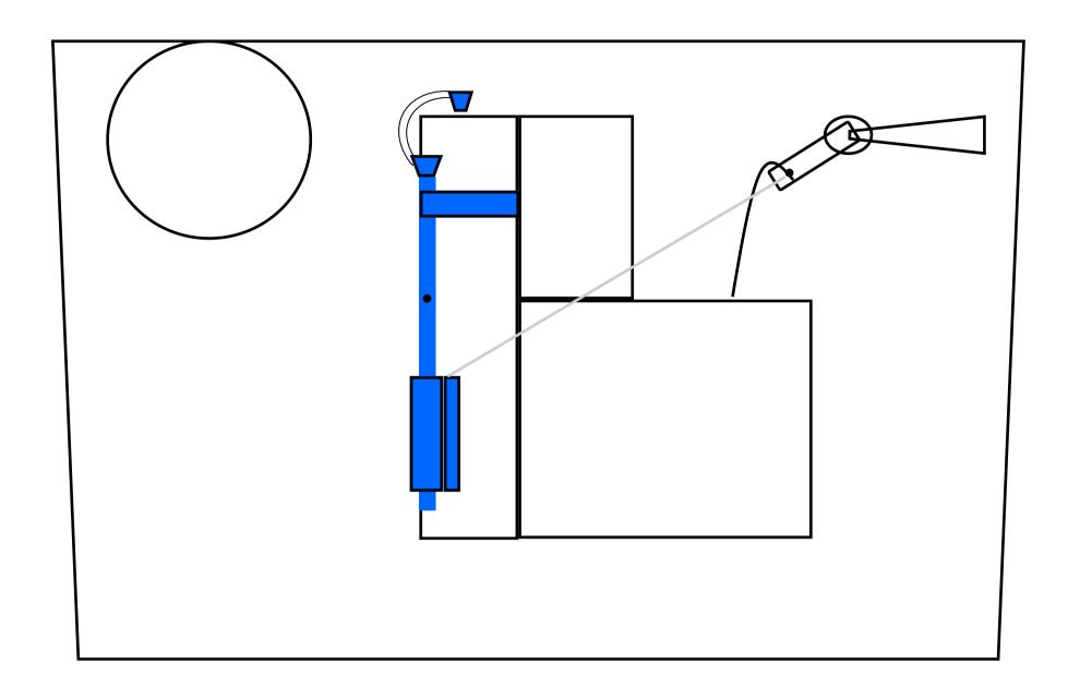
With handle depressed for half flush, occasionally a limited lift is available. Dependent on siphon type, cistern size, and flush handle. Extensive use has resulted in numerous installations with stretched cord and tightened knots. Resulting in poor full flush performance. Or no full flush at all.
